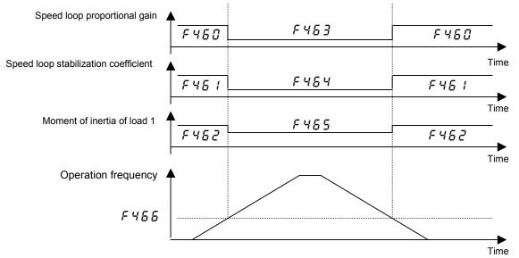
If the operation frequency is equal to or lower than the switching frequency (F 4 5 5: Speed PI switching frequency):
