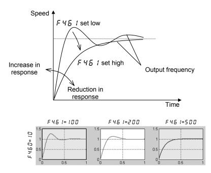
(2) Adjusting the setting of F 4  $\underline{B}$   $\underline{G}$  (speed loop proportional gain)
