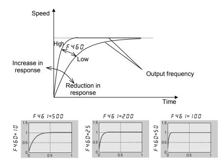
As described earlier in this chapter, the speed response is set to approximately 5Hz by default, based on the assumption that the inertia of the load is almost the same (1 time) as the inertia of the motor. Therefore, to increase the speed of response of 5Hz by a factor of K for a machine with inertia  $\alpha$ times as large as the inertia of the motor shaft, parameters  $F + E \Box$  and F + E i need to be set, as a guide, to the values shown below.
