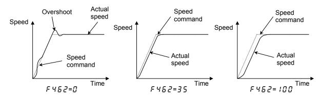
If you want to operate a machine with a low-inertia load at the highest possible acceleration/deceleration, you can increase the response by setting  $F \lor f \lor d$  to  $f \lor d$ .
